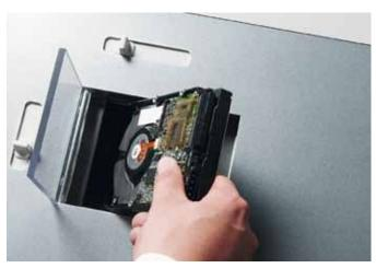
**FEEDING CHUTE WITH SAFETY FLAP** The electronically controlled, transparent safety flap is an important part of the SPS (Safety Protection System) package. The punching die can only be activated if the safety flap is closed.
